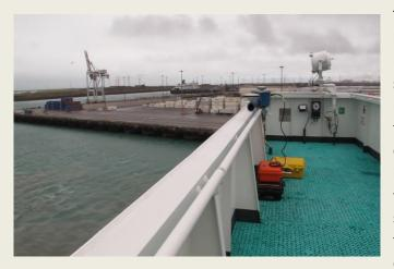
The motions of the vessel were recorded in 6 dimensions (3 translational and 3 rotational) at high frequency. During the survey, the rudder angle, the propeller rate of turn and the forces applied by tugboats were also captured. A survey carried out at full scale is always interesting because it reveals differences which cannot be predicted from model scale. For example, effects from wind and forces exerted by tugs may be quite different in reality.
