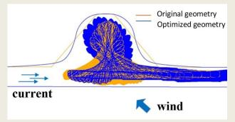
Based on a study carried out by <u>IMDC</u>, both a circular and a trapezoidal basin were selected, with two different sizes for each. The circular geometry is built on both sides of the channel while the trapezoidal is built on one side only. Real-time simulations with a ECMT class Va and a class Va+ vessel were then carried out in different current and wind conditions. The
