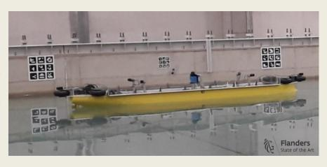
ships interacting with each other. For this type of experiments an accurate position measurement system is crucial. This is achieved by a combination of camera monitoring (towards so-called ArUco markers on the basin walls), LiDAR and gyro. The individual readings are then filtered to one position state record, which is made available for navigation routines on an on-board navigation computer. The system is expected to be production ready in spring 2022.
