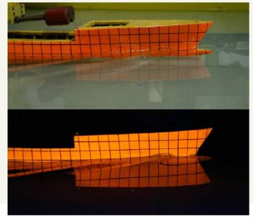
and a digital camera controlled via a laptop computer. The UV light emitted by the black lights is reflected by the fluorescent coating as visible light which is captured with a digital camera. An automated processing algorithm is in development at the Image Processing and Interpretation Division of Ghent University. Using this novel measuring technique, the dynamic waterline is evaluated not only much more accurately but also significantly faster.
