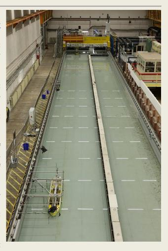
infrastructure, such as access channels, decreases. The focus of the PESCA project is to study the effect of parallel ship passages in high blockages at high passing speeds and close passing distances.
