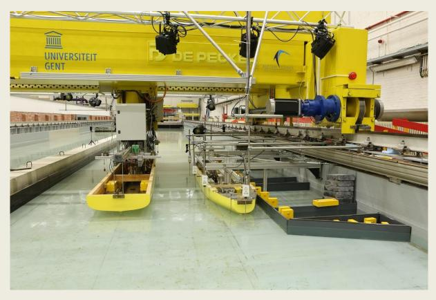
In the experiments, the blockage factor ranges from a situation in which the full tank width is used and 50% under keel clearance is present to a situation where the channel width is equal to four times the breadth of the passing ship with only 10% under keel clearance.
