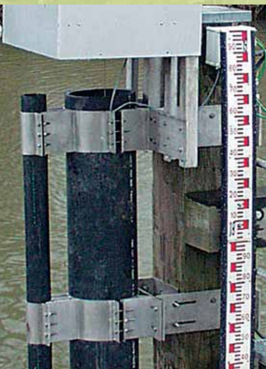
Stilling well with gauge
