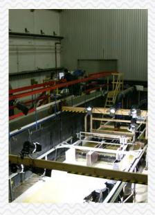
It is fitted with a carriage and can be used to calibrate measuring devices.
