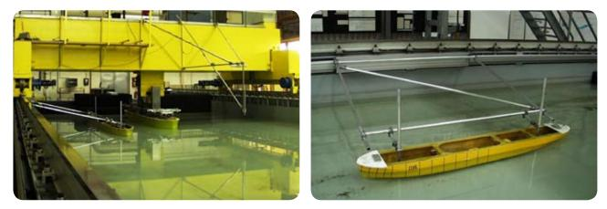
Auxiliary carriage for ship interaction tests
