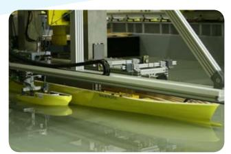
Ship interaction tests: tugboat and Container ship.
