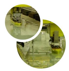
The ship passes along the built-in banks to measure the ship-bank interaction forces.
