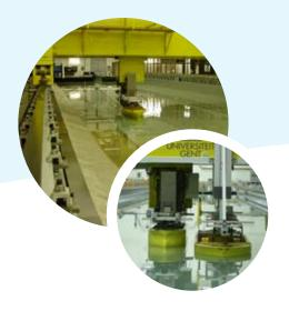
Scheur [fairway]. Through the waves the vessel will pitch, heave and roll. With larger vessels, this pitching and heaving response may be less, dependent on the wave spectrum, but the probability of touching bottom nevertheless increases on account of the decreased keel clearance and the greater effect of the rolling motion (due to waves, wind, bends) by vessels with a larger beam.
