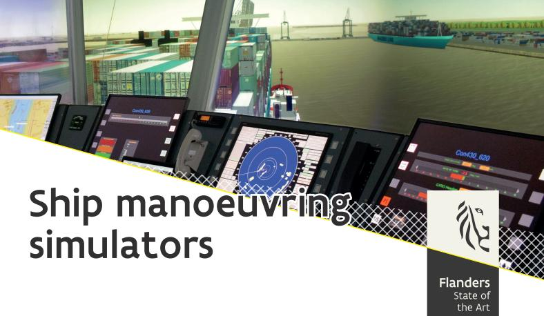
The ship manoeuvring simulator comprises various components. There is firstly the mathematical model. This is the calculating core behind vessel motions. Different forces act upon a sailing vessel: forces generated by the movement of the vessel through the displaced water, by wind, current, waves and other passing vessels.
